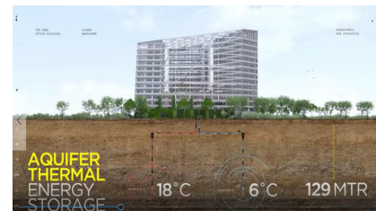
ATES (Aquifer Thermal Energy Storage) System.
